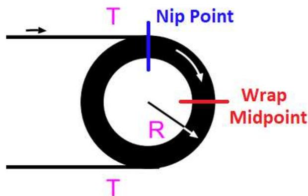
Diagram: Model setup showing nomenclature for Nip point and Wrap Point
