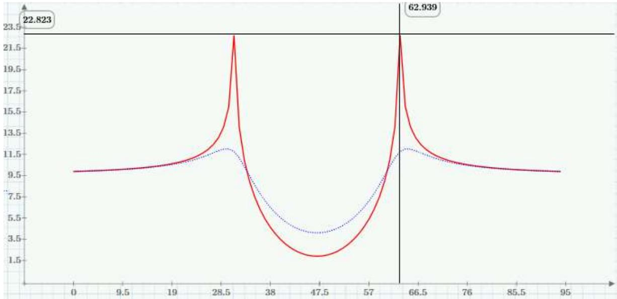
Plot: Tension (kN) within the steel cord cables at the nip point (blue) and wrap midpoint (red) vs Cord Number across the belt width
