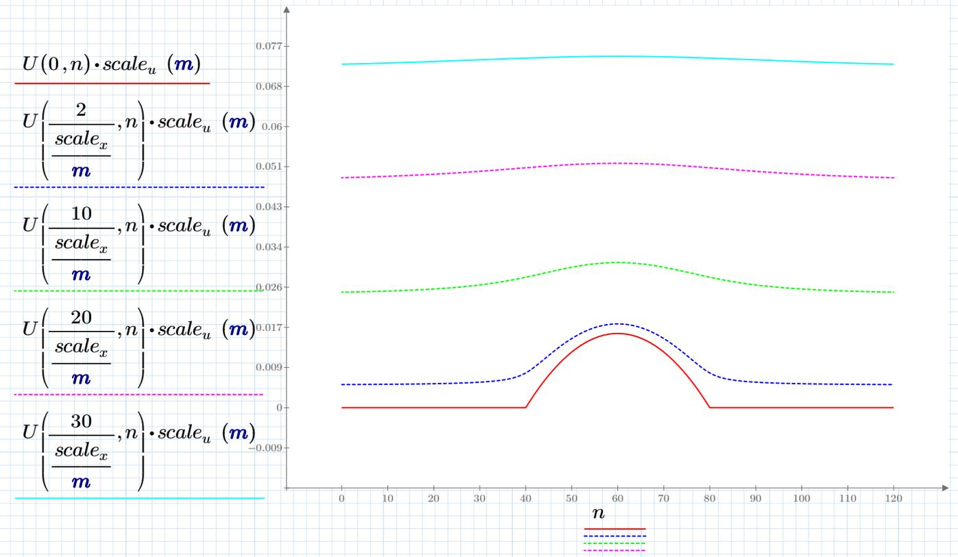
Cord Tension at Nip Point and Middle of Pulley Wrap vs Belt Width
