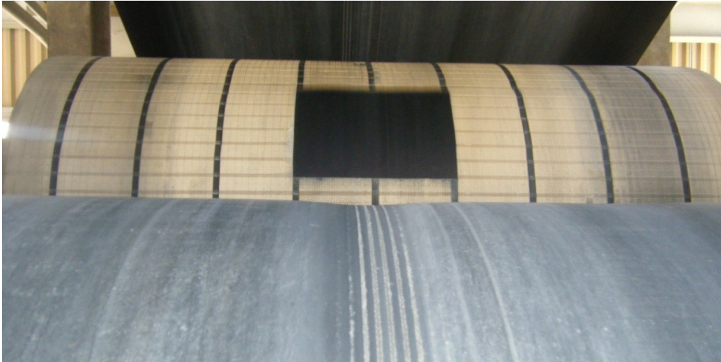
Figure 11. Bottom cover wear from ceramic lagging
