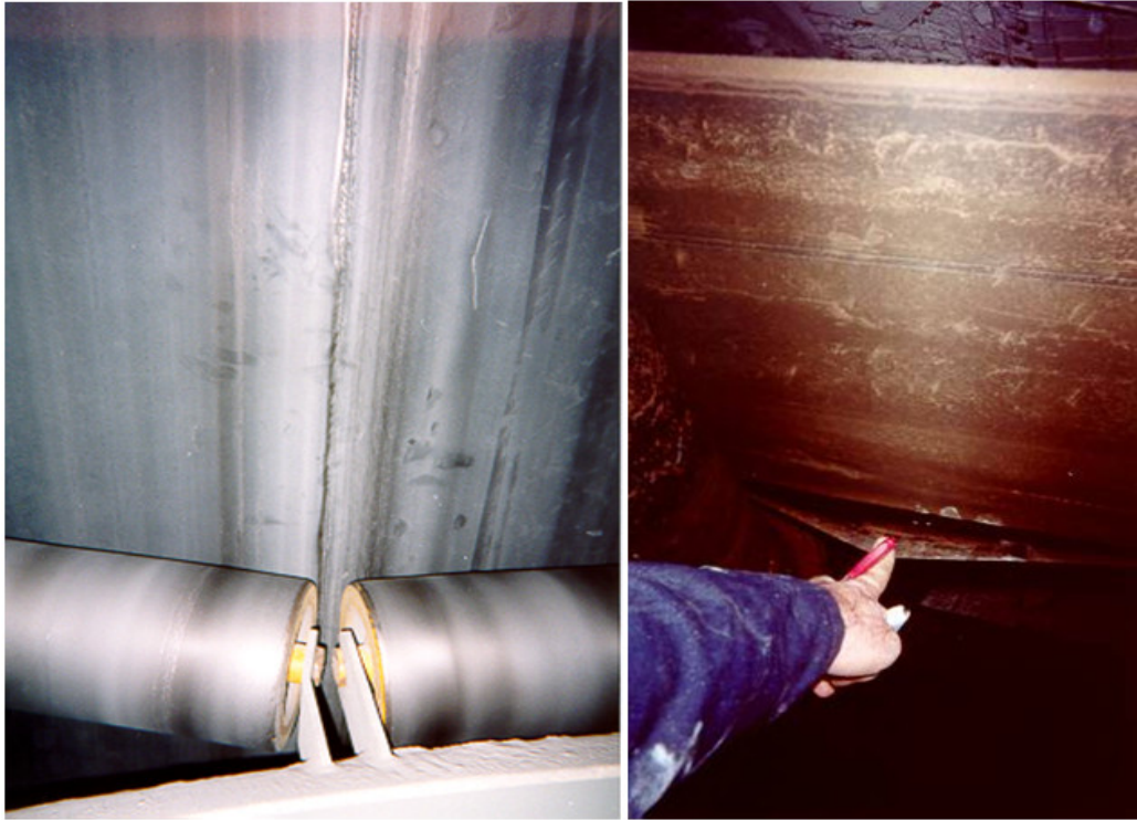
Figure 2 . Idler junction cover failure
