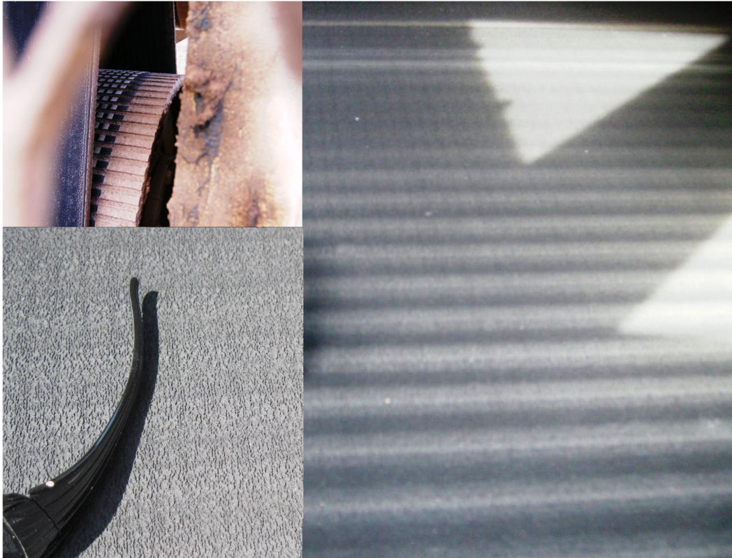
Figure 9. Belt cover wear from sharp ceramic lagging tile. The lagged pulley surface is shown in the upper left corner
