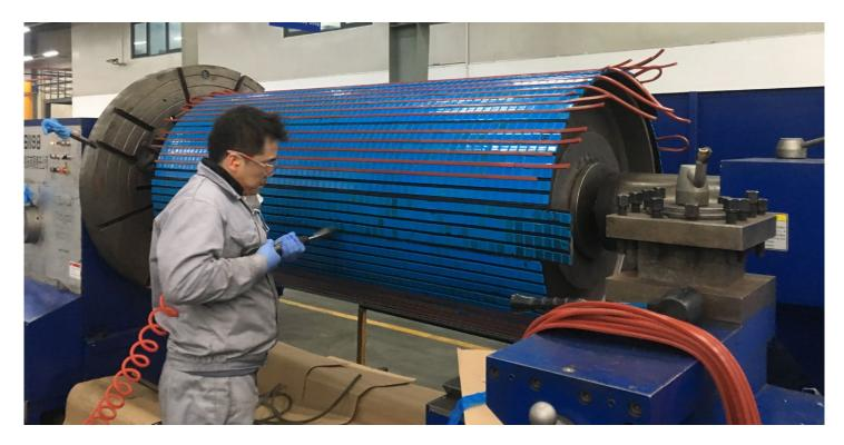
The two high tension bend pulleys with Elastotec HVPU were supplied to Oyu Tolgoi and put into service in early 2018. Greg Fogo (International Bulk Material Handling Director for Martin has visited Oyu Tolgoi to see the pulleys in operation and obtain feedback from the site maintenance personnel. Current operation is as expected with no sign of the buildup or excessive wear problems experienced previously.
