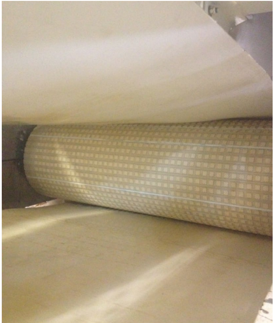
White ceramic lagging with white conveyor belt
