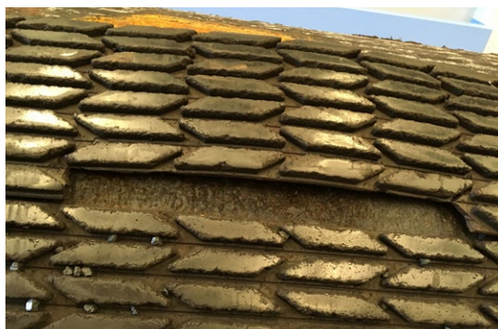
Photo #16 and Photo #17. Corrosion and lagging debonding at joints between cold vulcanised lagging strips due to water penetration.
