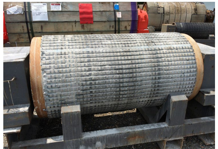
Photo #12 and #13. Severe lagging damage due to edge lifting and belt tracking.
