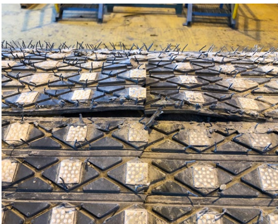
Photo #2. Cold vulcanised lagging failure due to debonding under load at low temperature.
