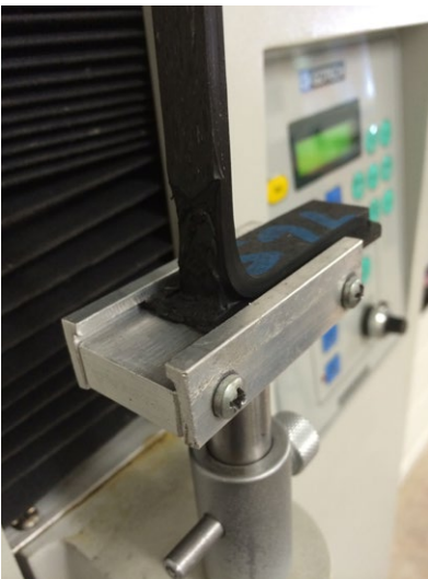
Photos #4, #5 and #6. 100% Rubber Tear bond obtained with hot vulcanised lagging application and tested on EVERY Elastotec lagged pulley.
