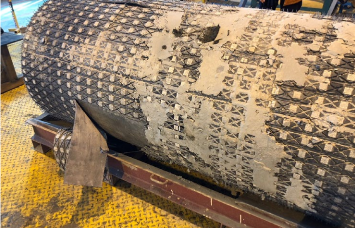
Photo #3. Cold vulcanised lagging failure due to debonding under load at low temperature.
