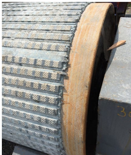
Photo #12 and #13. Severe lagging damage due to edge lifting and belt tracking.
