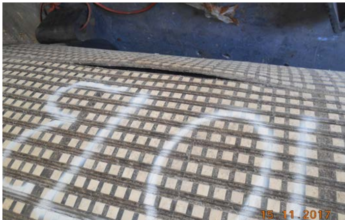
Cold bonded lagging lifting at the joints after long term storage.
