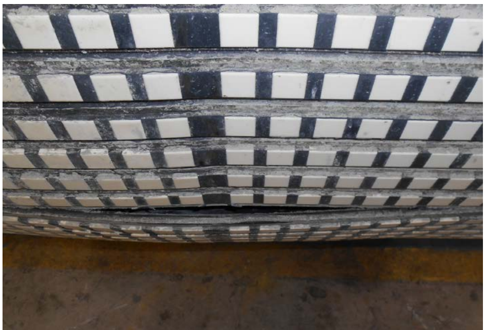
Spare pulleys stored for several years but not put into service due to cold bonded lagging debonding
