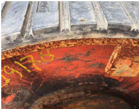
Hot vulcanised lagging – no edge lifting after exposure to wet and corrosive conditions.
