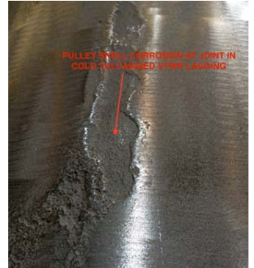
Corrosion of the pulley shell along the joint between two strips, this can reduce shell thickness and make the pulley unsuitable for service.
