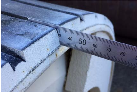
Cold bonded lagging opening up at the joint between strips during storage.
