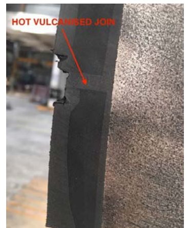
Hot vulcanised join – will not open up.
