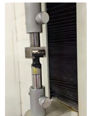
Image#7 - Tension pull adhesion testing
