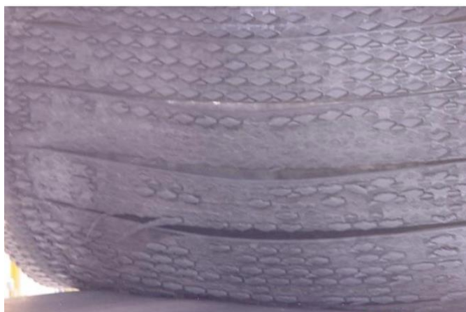
FIGURE 1 - Picture of a failed lagging application showing both lagging abrasion and delamination.
