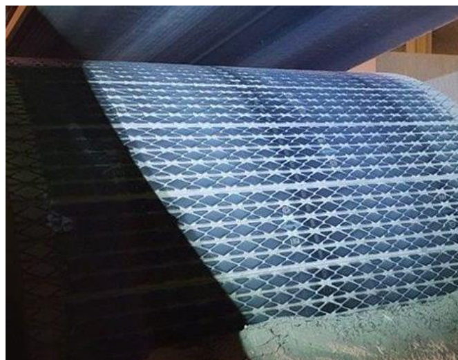
FIGURE 3. DRIVE PULLEY IN OPERATION WITH DIAMOND LAGGING.
