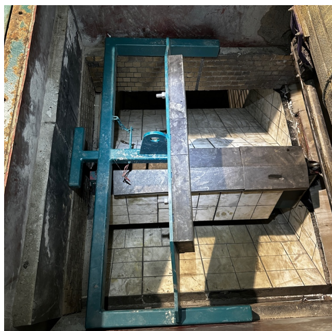
MAIN IMPACT ZONE WILL HAVE A HIGH INTEGRITY ZTA CERAMIC CALLED ZTA WHICH WILL FURTHER DECREASE WEAR IN THESE AREAS.
