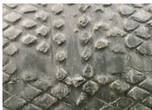
6MW Drive NSW, Australia, Melting of rubber
