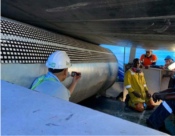
Elastotec ceramic lagging being applied on conveyor with Elastotec supervision and training
